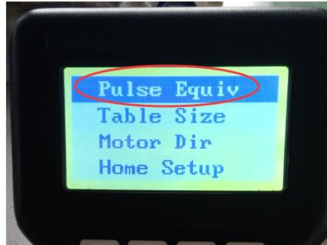
Press ORIGIN menu, you will be guided to pulse set up, now input pulse value for x, y and z axis: X=120 Y=120 Z=400.
